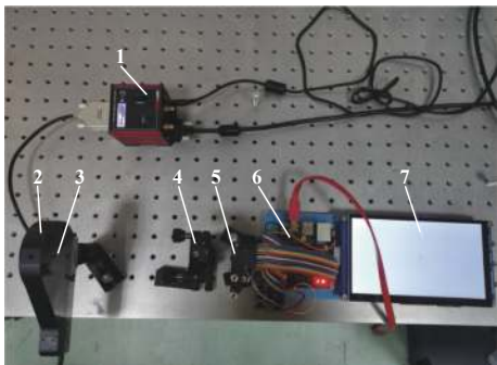
1.驱动器; 2.电动精密旋转位移台; 3.光栅片; 4.物镜组; 5.CMOS 相机; 6.Zynq; 7.LCD
